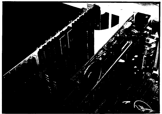
Photo 6: To aid in my initial development, a Zscan-8000 emulator is plugged by a ribbon cable into the Z8001 socket on the Trump Card. In emulation mode, the Zscan-8000 can run diagnostic programs and exercise all functions of the Trump Card at 4 MHz. Hardware debugging is greatly simplified because all sections of the hardware need not be working to use the emulator.
